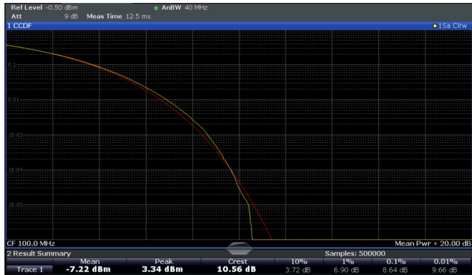
Fig. 3-14: CCDF measurement results for BTS mode
